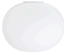
Ceiling mounted lamp providing diffused light. Diffuser consisting of an externally acidetched, hand blown, flashed opaline glass and of a die-cast aluminum threaded ring nut with alodine plating finish. 30% fiberglass reinforced injection-molded polyamide ceiling fitting; gray painted die-cast aluminum diffuser support.
